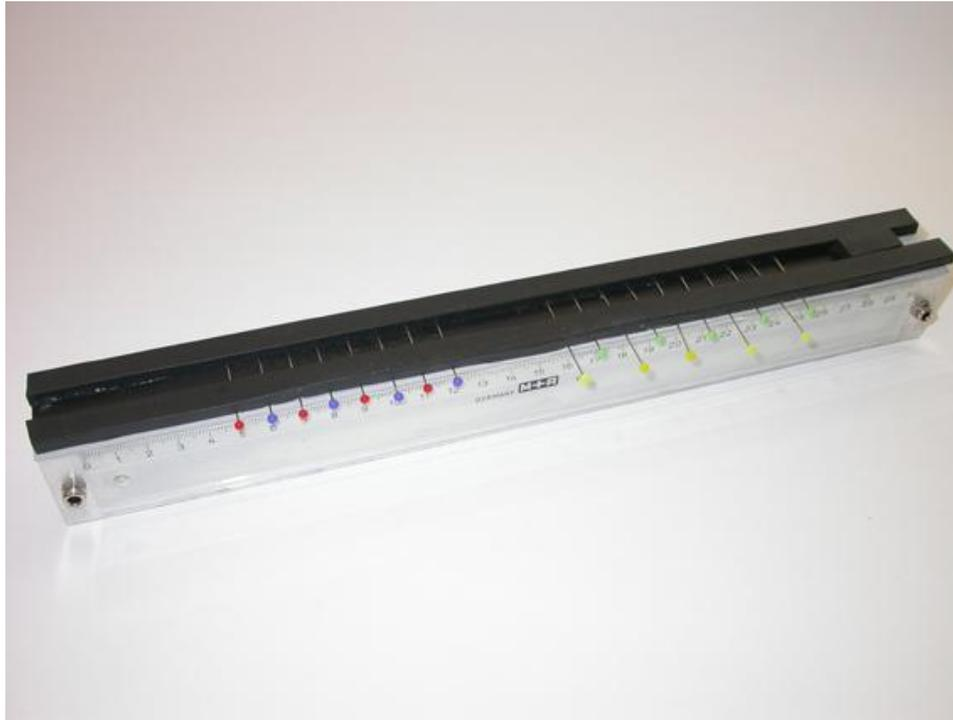
*Supplementary figure 1:* Assembled earthworm cage. The aluminum U-profile is covered with foam rubber through which pin electrodes are pushed.
